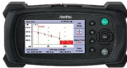
Micro OTDR MT9090A 1310/1550/1625nm 38/37/35dB SCAPC + sac /C Modele MU1004
